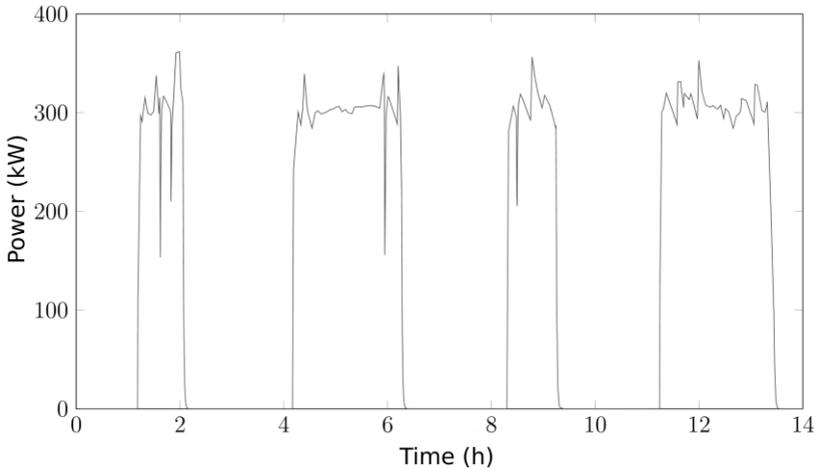
Fig. 2.3: Residual engine power during well stimulation process [1]
