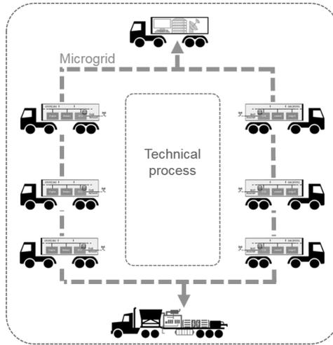
Fig. 3.1: Mobile industrial fleet connected to an islanded microgrid [2]
