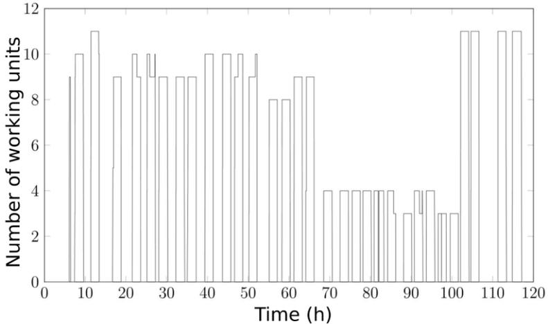
Fig. 1.2: number of working units during well stimulation process [1]
