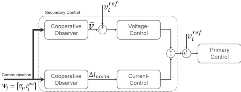
Fig. 3.4: Cooperative control system on the units of the mobile industrial fleet
