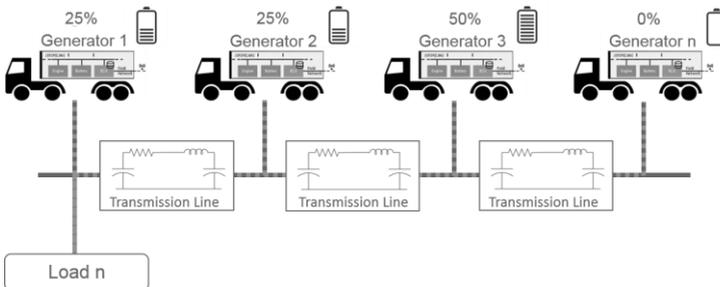
Fig. 3.2: Load sharing in microgrid applications [2]
