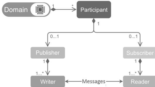
Fig. 4.1: Data Distribution Service communication entities of the specification [4]
