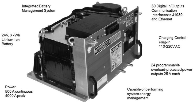
Fig. 2.1: Power Module of Engine Standby Controller
