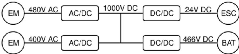
Fig. 2.4: Schematic setup of the pump unit board grid [1]
