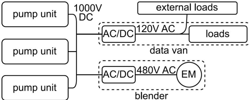
Fig. 2.5: Schematic setup of the fleet micro grid [1]
