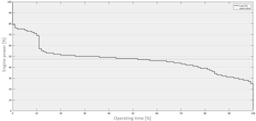
Fig. 2.2: Load Factor of pump unit with ESC
