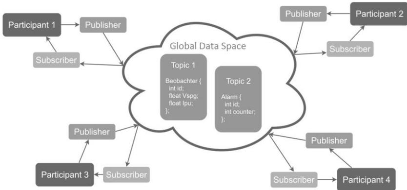
Fig. 4.2: Network design based on the data distribution service specification
